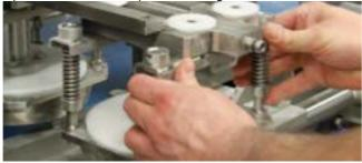
Rounded edges and fully open covers on both sides of each unit are applied throughout the system. The best possible accessibility of the process is achieved by optimizing the space between the working stations. Tools that are attached to the machine, are mounted with standoffs. With a minimal distance of 1 inch for cleaning purposes. Lightweight safety covers with extra handles enable ergonomic operation.
