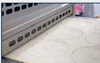
4. Product cutting: cutting products out of the dough sheets. Multiple shapes, sizes and rim press are possible.
