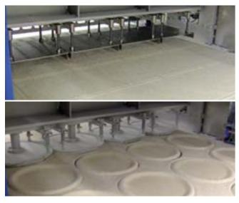
Various product shapes can be cut by the same cutting module and cutting change-over tools.
