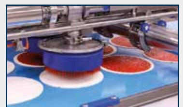
6. Sauce depositing: Tomato sauce (or other sauce) is deposited on the pizza base. Various methods are available, for instance showerhead depositing and stripe depositing.
