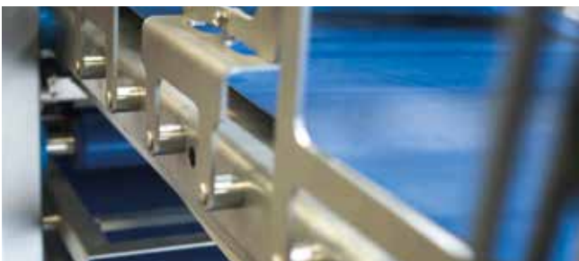
Accumulation of dirt and dust is reduced due to the application of stand-offs.
