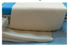
The belt with the dough sheet moves back and forth above the next conveying belt. This is an asymmetric lamination system suitable for soft dough with no restrictions regarding laminating width.
