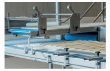
A guillotine cuts the dough sheet into regular rectangular sheets which are then stacked on top of each other. This flexible symmetric system lays even and uneven layers. Suitable for soft doughs with no restrictions regarding laminating width.
