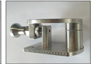
Quick release mechanism for fast and easy change overs
