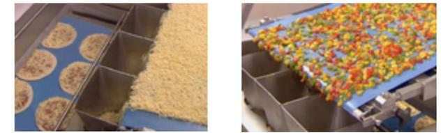
Fixed shape travelling hoppers for 'indexed' pizza topping systems leaving pizza rim free of topping. This system doesn't need a recirculation system. Change-over parts are needed when different sizes or shapes need to be topped.
