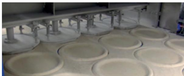
*Various product shapes can be cut by the same cutting module and cutting change-over tools.*
