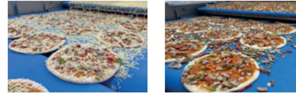
Product size flexibility is offered with this system, as several pizza shapes and sizes can be topped on the same system without change-over parts. This system offers the highest output and reliable strewing accuracy through an innovative algorithm. A recirculation system is integrated to recirculate the topping material.
