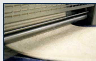
**2. Reduction stations:** reduces the dough sheets thickness to the final thickness.
