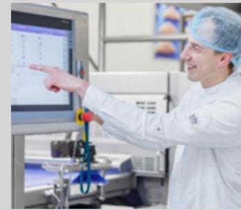
Great care is given to the user interface of the 22-inch touch screen. Its position can be effortlessly tailored to the preferred working height. The control platform facilitates seamless OMAC-based data exchange with neighboring third-party equipment. Advanced data processing empowers real-time monitoring and the fine-tuning of equipment efficiency.
