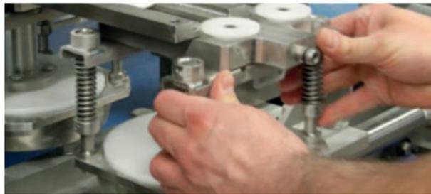
*Efficient, error free operation and tool change-over is realized by applying Unique Fit Tooling. Because of the lightweight and more compact tooling, handling and detaching the tools is as easy as possible and can be done by one person.*
