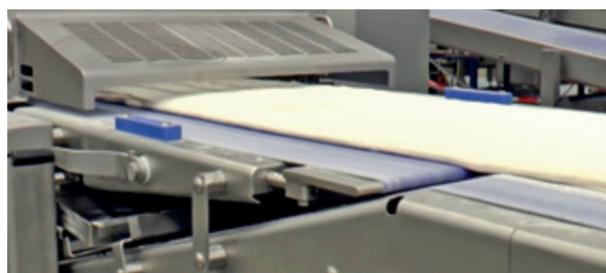
*Elimination of falling heights: by minimizing the transportation height throughout the production line, it results in a stable and relax dough sheet.*
