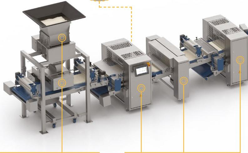
The dough batch is processed in two steps through low stress pre-sheeting systems into a continuous high quality dough sheet.
